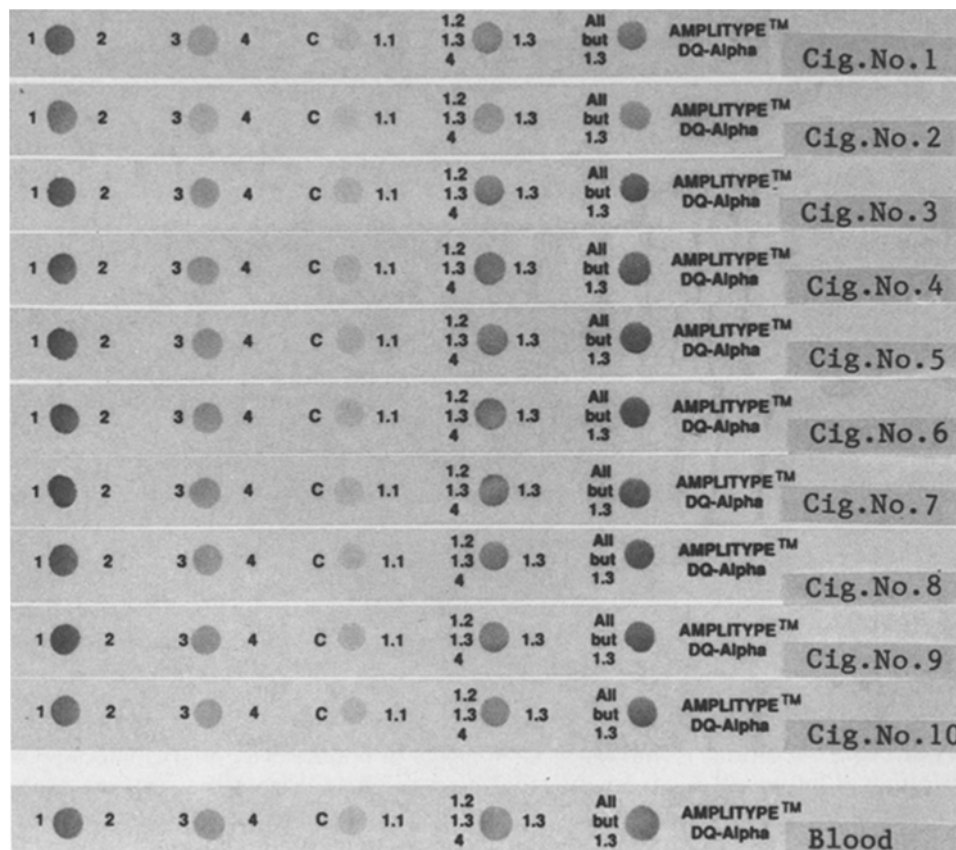
Fig. 2. Typing of HLA-DQ alpha locus after PCR using reverse dot-blot strips. DNA extracted from the butts of 10 cigarettes smoked by one individual (Cig. Nos. 1–10) yielded results identical to the control blood sample (HLA-DQ alpha Type 1.2,3)
